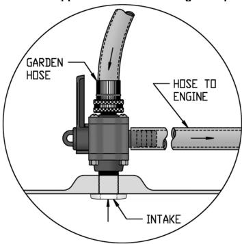
Regular fresh water flushing will extend the life of your engines cooling system. Now you can winterize easier and flush your engine regularly without the cumbersome changing of hoses, using pumps or other equipment. This Marelon® system makes it simple and fast.
